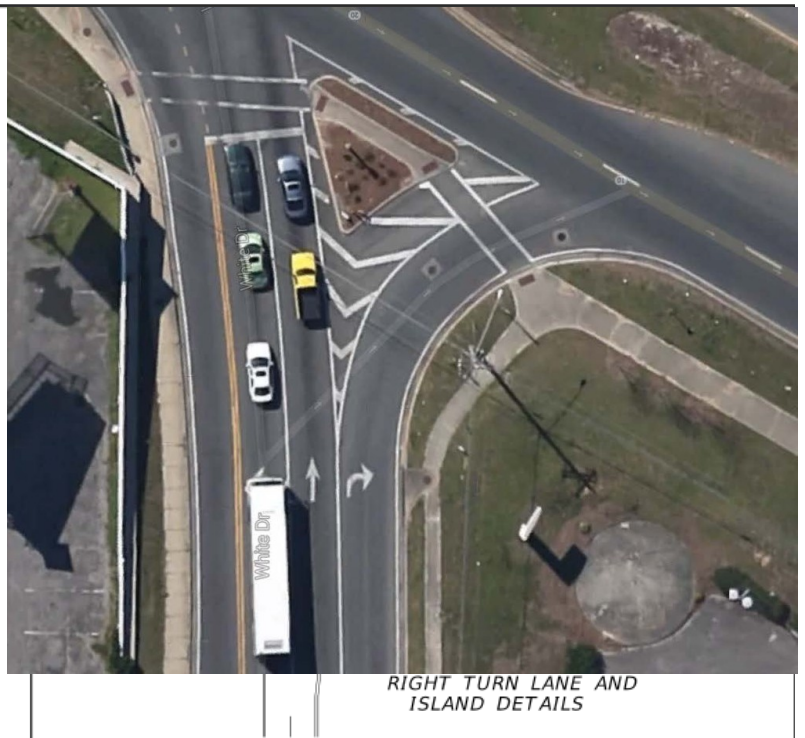
Florida DOT Standard "17346 - Special Marking Areas". Source: FDOT Design Standards, 2014
