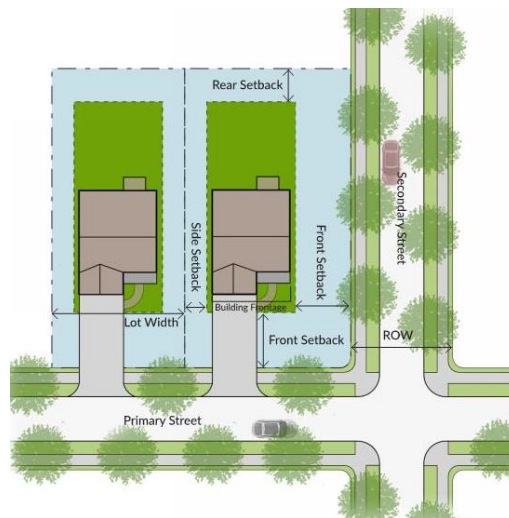
FIGURE 4-4 LOT WIDTH, BUILDING FRONTAGE, AND SETBACKS
